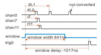
The trig0 -1017 ns is the virtual start for the data. Channel resolution is selected to 1/64 ns (15.6 ps) The generated event structure looks as follows (channels are in arbitrary order):
