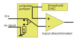
"P" means jumper position near to front panel, then input is terminated.
