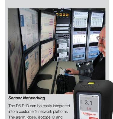
Reachback files are given as an output by the detector for integration. This enables a single control point for multiple integrated sensors, rather than using each one individually.
